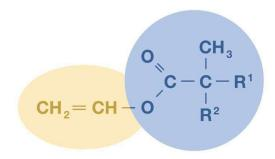
R<sup>1</sup> and R<sup>2</sup> are alkyl groups containing a total of 6 carbon atoms. VeoVa 9 Monomer, a low viscosity liquid with a typical mild ester odor, is a very attractive monomer for the manufacture of polymers through reactions of the vinyl group. It imparts a combination of high polymer hardness (high glass transition temperature), hydrophobicity and very good chemical and UV resistance.
