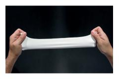
Hexion developed a vinyl-modified acrylic resin based on vinyl acetate, VeoVa 10 vinyl ester, and butyl acrylate. This resin was tested in a formulated elastomeric roof coating against a leading all-acrylic emulsion.
