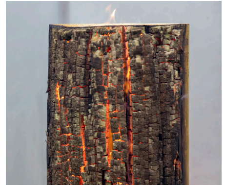
Pole without ArmorBuilt protection
