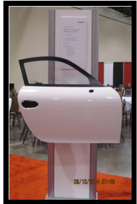
Assembled door body of carbon fiber composite made with Momentive Specialty Chemicals epoxy resin system
